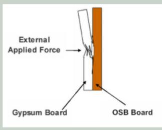
This illustration shows the main function of chipboard in making every element strong when added as a membrane. It is systematically placed between
