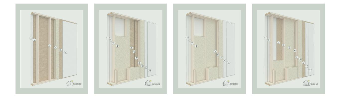
In all types of duplexes, terraced houses and apartment buildings, the walls between the homes and apartments can be anti-fire. We recommend using fermacell instead of cypsum, as it gives strength and rigidity to the building, as well as making the wall more soundproof.
